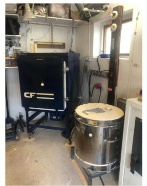
thermocouples from Wish and Banggood. I installed second thermocouples (red) into each of the ovens and wired them up to the new PIDs, then proceeded to compare the temperatures these parallel systems reported compared to the original controllers still attached to the ovens.
