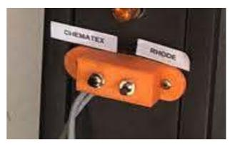
But I have two ovens. Sure, I can pug either one into the controller, but since every oven has different PID parameters I would have to change the parameters and restart the kiln-controller subsystem each time I changed ovens. That would be a pain.
