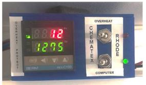
OK, so now I had two ovens with two thermocouples each, and DPDT switches in my controller box that flipped the MAX31856 interface card between the original thermocouples in one or the other oven. That's great, *but now I had to figure out the actual powering and control of the power to the ovens.*
