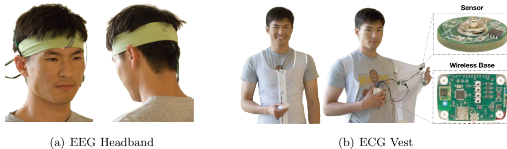
Figure 2.3: Wearable devices using non-contact electrodes. Picture from (4)
